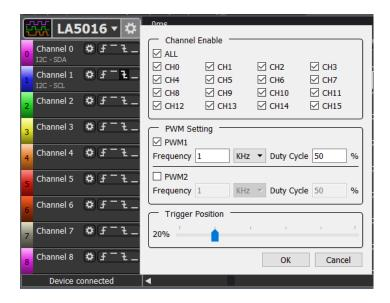
As is shown in the right figure, the channel settings window of LA1010 are a little complicated. Because the maximum sampling rate is related to the number of the channels enabled, we provide several quick selections in the settings window, to make the channels switch rapidly among the sampling rates that are available in LA1010.
