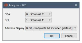
1<sup>st</sup> item, the channel used for SDA signal (data)
