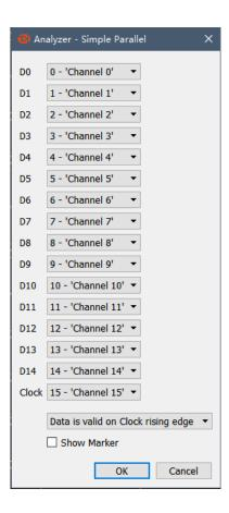
1<sup>st</sup>-15<sup>th</sup>items, the channels used for 15 parallel ports.
