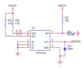
Pin 27 and 28 are always reserved for an ID EEPROM on the Raspberry Pi. Independently which card you use. It's useless for most application. If you want to use this function, you need to solder the IC, resistance and capacitance by yourself.
