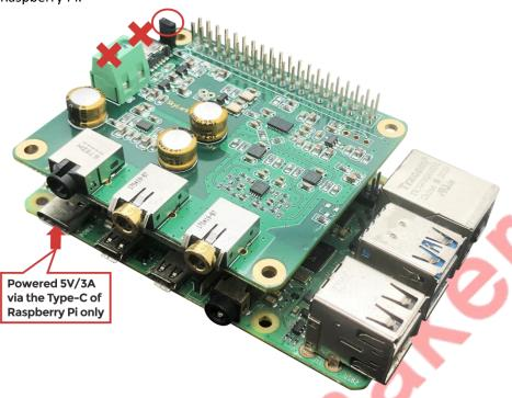
3) Remove the jumper, Power the Raspberry Pi and DAC hat separartely. This way can be properly isolated the Raspberry Pi and DAC hat. The dac have only need 5V/1A independent power supply. This is the best power supply way for music quality.
